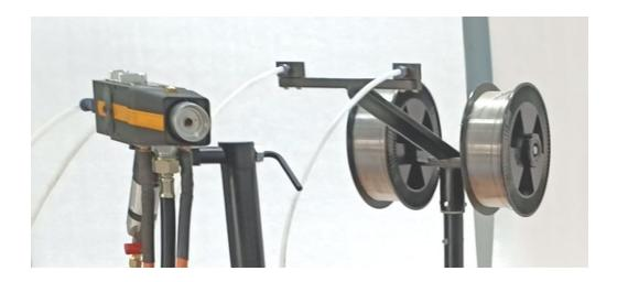
Arc spray system is offered with wire reel stand for holding the plastic wire spools and allows easy & smooth rotation of spools while arc spray coating is going on, thereby offering consistent and uninterrupted wire discharge from the spools. On the wire reel stand a push-in connector is offered to fix the Teflon tubes in the connector.
