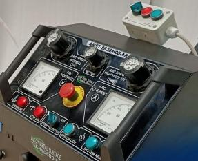
The offered Power source is designed to meet the requirement of electric arc technology of DC voltage with integrated control and ergonomic as well as user friendly control panel. The start & stop of the arc is achieved by pressing lever of air motor thus offers dead-man handle for safe working operation stopping the gun, if dropped down.
