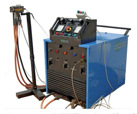
Offered twin wire arc spray system; Model :WST-8830/600-AR combines typical features of the modern arc spray technology. The offered system operates on Pull Type principle wherein the wire is pulled by the electric arc gun roller which is driven by a pneumatic air motor.
