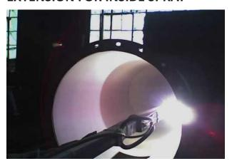
For years, the arc spray process has been limited in its ability to reach internal diameters. The development of ID arc spray extension has been a major leap in improving process technology.
